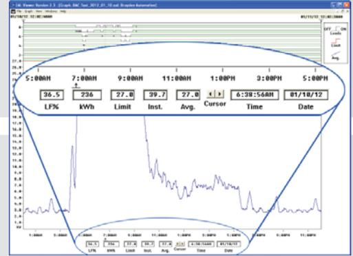
Detailed information of each log file's data points are displayed at the bottom of the Graphing Window.
