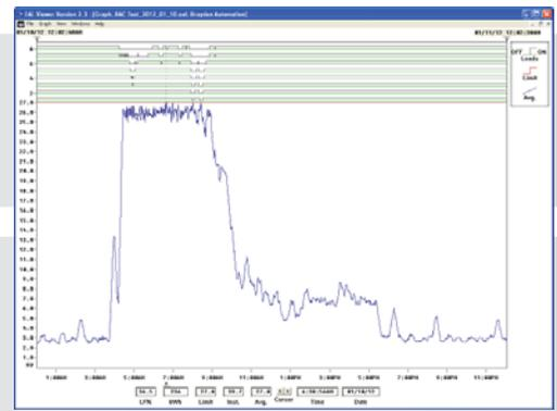
The Graphing Window allows graphic display of load profile and control information.
